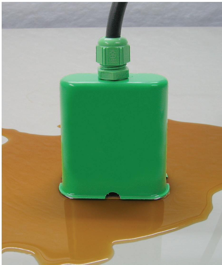
The Jola "Pumpswitch" device is a conductive floor electrode with integrated evaluation electronics and a delayed switch-off power relay for the direct switching of a flat suction pump.
