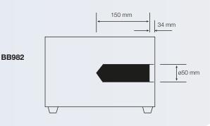
The BB982 Portable Blackbody Calibration Source allows for calibration of non-contact infrared thermometers over the temperature range -10°C to 80°C.
