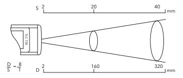
Please ensure that the object being measured is larger than the distance between the two laser points. The smaller the measured object is, the closer you must be to the object.
