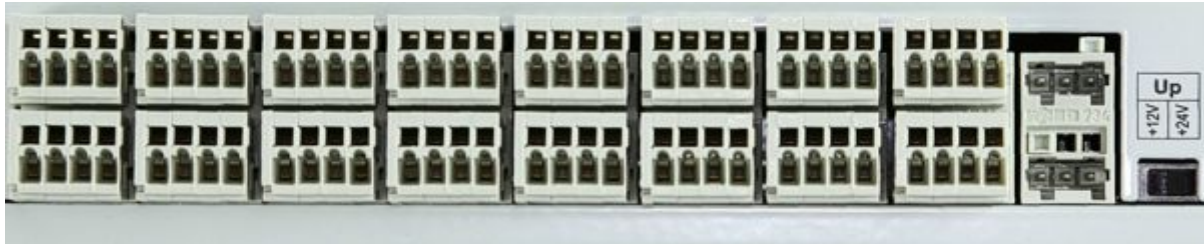
Figure: data logger inputs with switch 12Vdc/24 voltage power supply for connecting sensors. Serial input RS485IN a surcharge.
