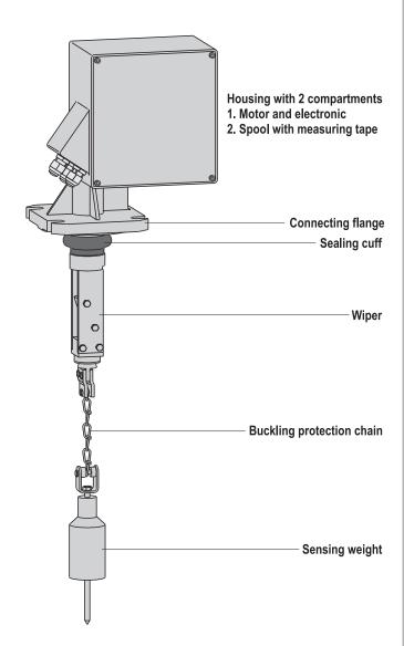
**Sensing weight** has to be suitable for the chemical characteristics of the bulk good and the process temperature within the bunker or silo.
