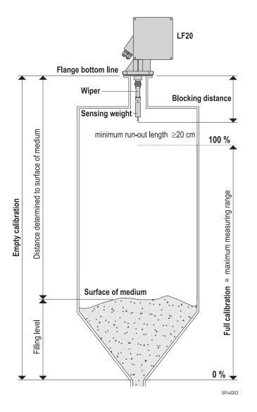
The measured value is the distance between the flange bottom line and the surface of the medium minus the block distance. (see figure "measuring categories") The filling level is calculated taking in account the calibration values entered, e.g. silo height.
