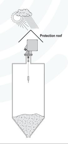
For use in external areas being exposed to climatic conditions we recommend the weather protection hood or an additional protection roof.
