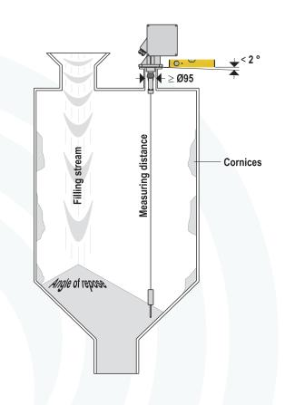
Select the mounting location on the bunker or silo roof in such a way that falling product during filling or collapsing cornices cannot spill the sensing weight and cannot damage the measuring tape.
