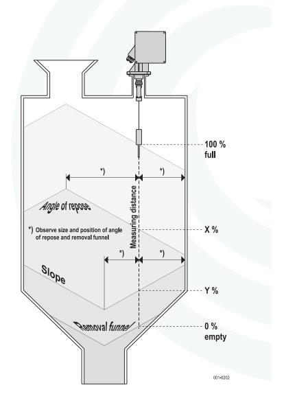
During the up and down movement of the sensing weight the relay output of the LF20 can additionally emit pulses according to the length of the rolled out measuring tape. These pulses can be recorded by a process control system or an electro mechanical counter.
