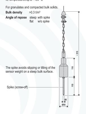
9.**G** Bag sensing weight Polyester and stainless steel for temperatures up to +150 °C
