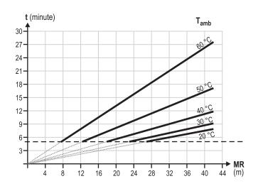
The minimum time  $(t_{minute})$  for one measuring cycle (time between two measurements) is dependent on the ambient temperature  $(T_{amb})$  and the measuring range  $(MR_{meter})$  and must not be undershoot in all types of measuring.
