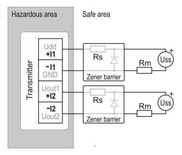
Loop resistance value Rc = Rm + Rs + resistance of wires shall fulfill the condition  $Rc[\Omega] < 40 \times Uss[V] - 360$ .
