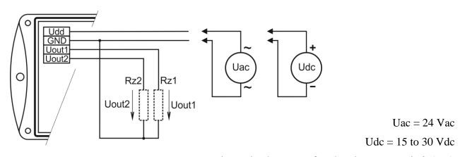
maximum load current of each voltage output is 0.5 mA
