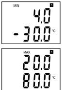
Range and type of value for output 1 (current loop II = symbol ",1" on display). Type of value, assigned to output 1, is indicated by displayed unit (here  $^{\circ}C$  = temperature). Upper line displays current value corresponding to measured value (lower line). Here 4 mA corresponds to -30  $^{\circ}C$ .
