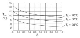
Graph showing the minimum measurable object temperature (T<sub>min</sub>), determined by surface emissivity (ɛ) and sensor temperature (T<sub>S</sub>).
