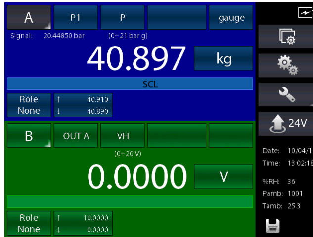
Figure 78 – Channel with active Scaling function
