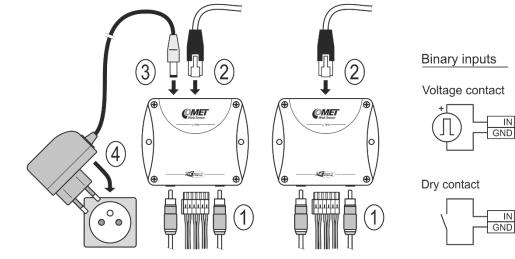
Binary inputs terminals connection procedure:
