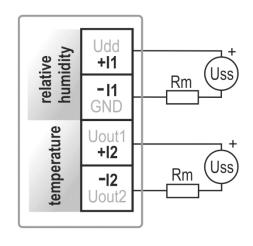
The loop resistance value Rc = Rm + resistance of wires shall fulfill the condition  $Rc[\Omega] < 40 \times Uss[V] - 360$ .
