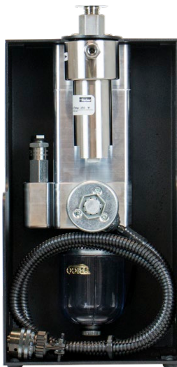
Figure 8.9.2 - Automatic Contamination Prevention System
