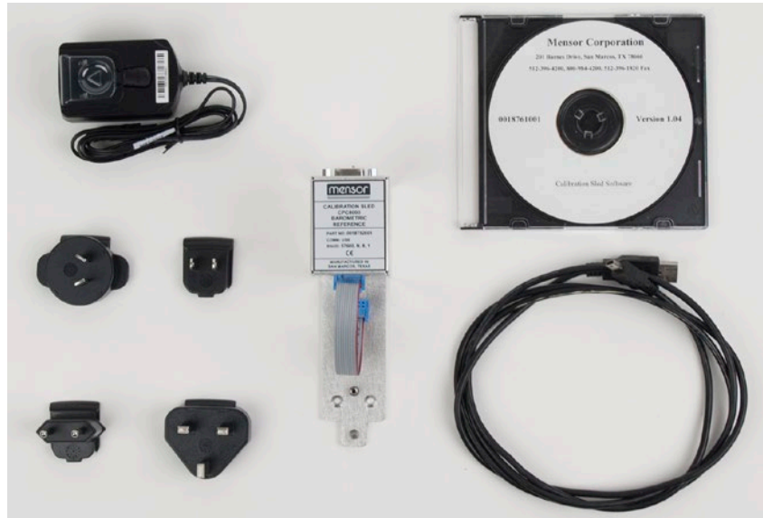
Figure 8.5.2 - CPA2501 Barometric Reference Cal Sled Kit
