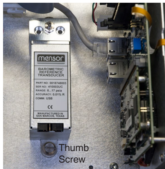
Figure 8.5.3.2 - Internal Barometric Reference
