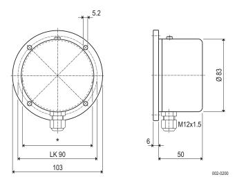
\* Hole-Ø in the vessel max. 80mm
