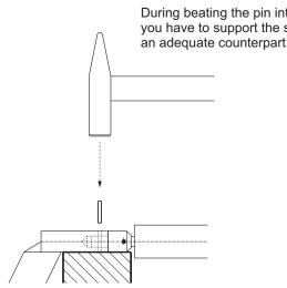
During beating the pin into the shaft, you have to support the shaft with an adequate counterpart.
