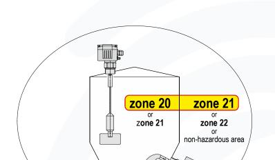
The "X" behind the number of the EC-type-examination certificate means that the device can be installed in the walls of silos, vessels, machines, filters etc. when the inside is classified as zone 20.
